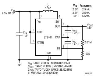
Figure 5. 34V Bias Supply Using the LT3464
